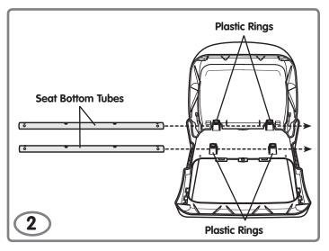
Slide a seat bottom tube through each set of plastic rings on the seat bottom.
